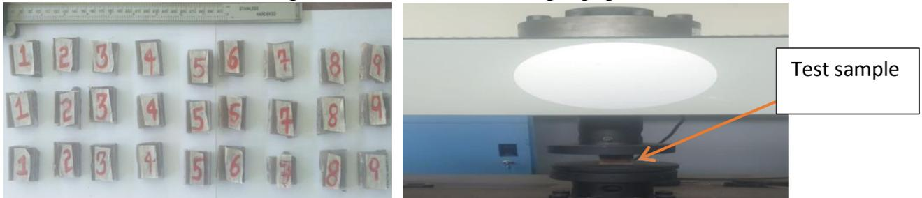
Figure 6 a) Compressive strength test samples b) Setup for compressive test The compressive strength can be mathematically equated by the equation below [24].
